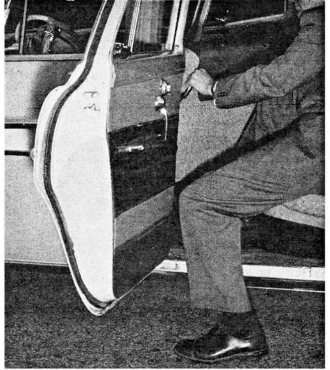
Doors open to nearly 90 degrees for easy entry, exit. Car is almost 2 inches lower than '54, headroom is only 3/4-inch less
