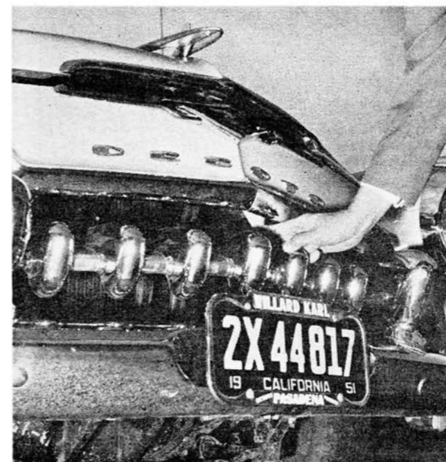
Grille remains customizers' gold mine (they like the "teeth"), hides hood latch. Chrome is lavish per sales demands
