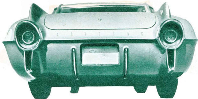
Pontiac's Strato Star features new way of enclosing dual exhausts, also serves as protection. Rear end treatment gives feeling of enclosed undercarriage
