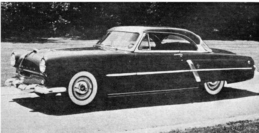
One of several mechanical prototypes developed from a '53 Lincoln hardtop for testing chassis components of new Continental, which will have similar height and length
