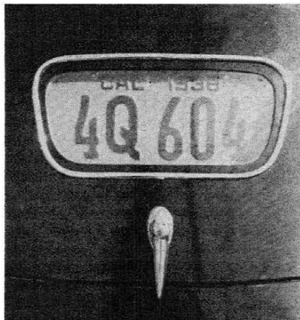
First inset license plate was fashioned by Frank Kurtis in 1936 on an early Airflow DeSoto, was widely copied later.
