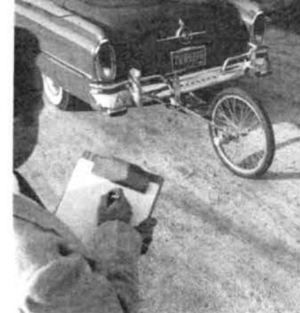
Fifth-wheel checks under acceleration indicated reworking of automatic transmission has smoothed out gear changes.
