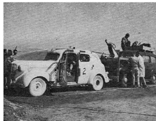
Crash car and control car are in position preparatory to another test from which evidence will be gathered by scientists.
