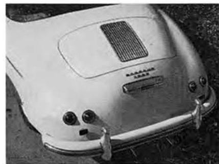
The rear-mounted flat-4 engine is air-cooled.
