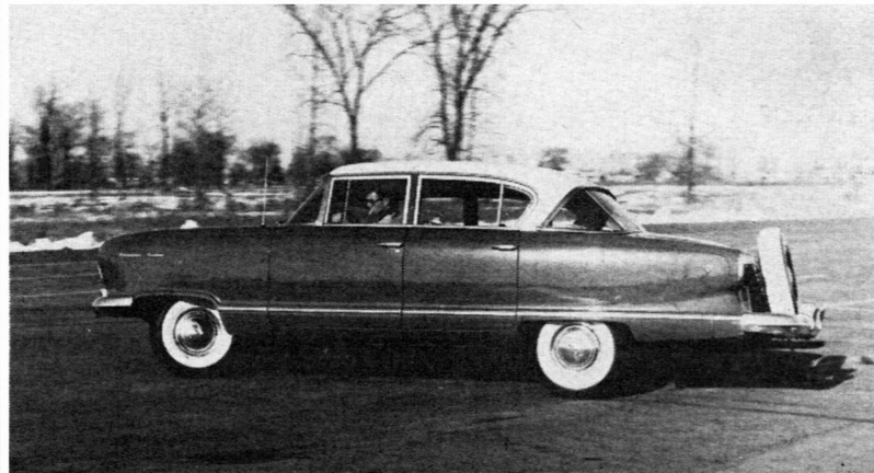
Nash heels as driver bends it into a hard corner. Unit frame design makes car exceptionally rattle-free, gives it good safety rating.
