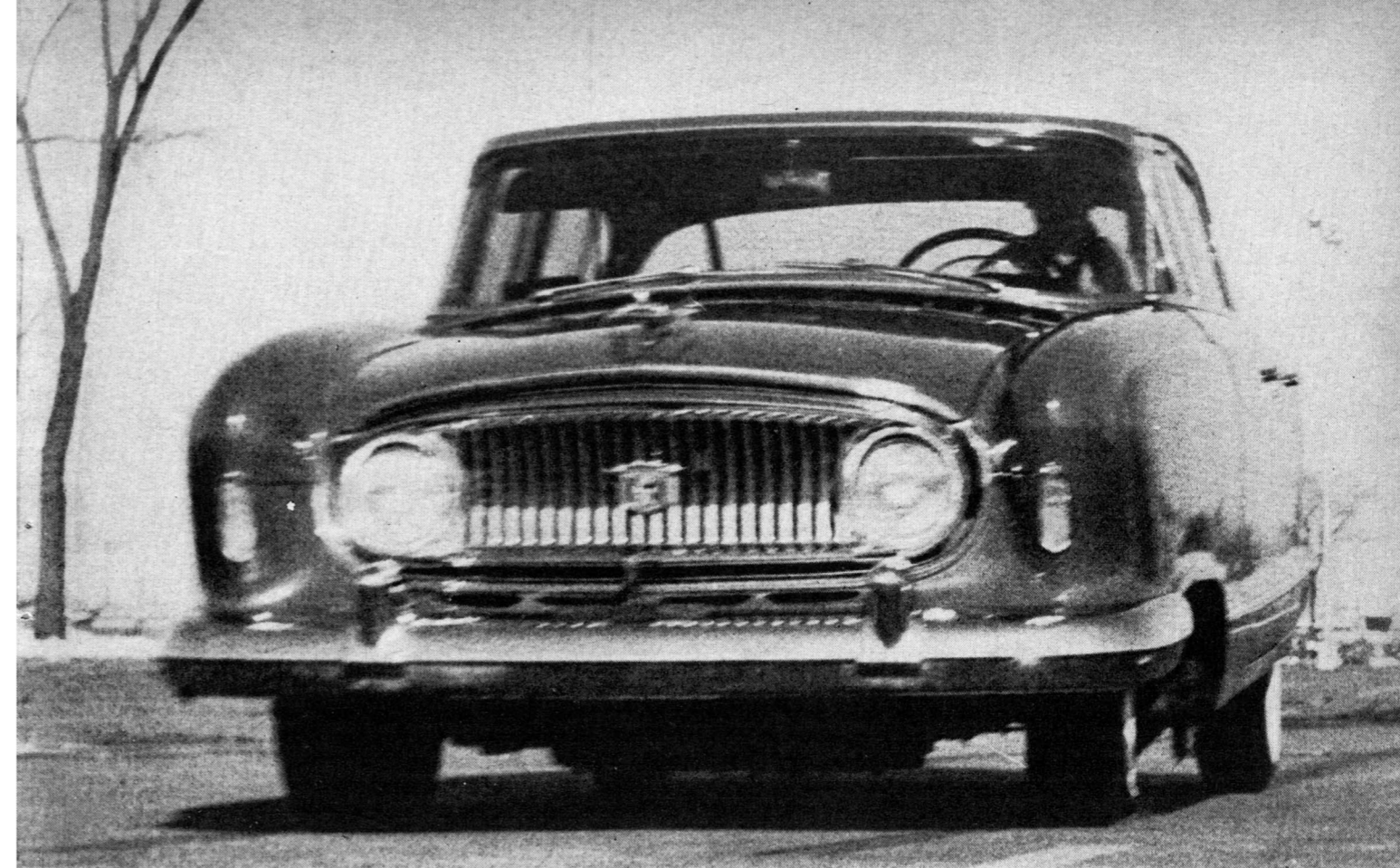
Front end has normal dive under hard braking, but held a straight line. Note how the headlights are now inboard in grille.
