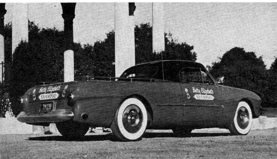
Passenger car body (1950 Ford two-door) formed the basis for this novel pickup, by Joe Bailon, of Hayward, California. A five-inch sectioning operation, stiffening of side panels were the principal tasks he performed.
