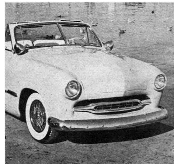
Typical custom touches of early Fifties are Frenched headlights and floating grille, worked into this '50 Ford by Bob Travers of Oakland.
