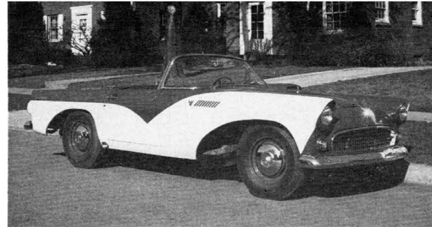
Thunderbird has wheel cutouts enlarged and reshaped to give lower, racier appearance. Next step planned by owner is a Ferrari-type grille and fiberglass bucket seats.
