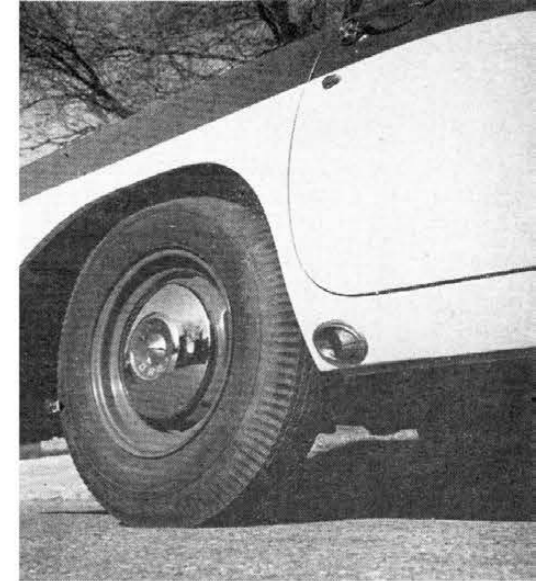
Exhaust pipes have been brought out through panels below rear edge of doors.
