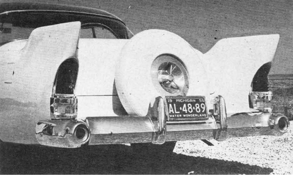
Rear quarter panels borrowed from a Lincoln had high-flying fins added before grafting onto '54 Buick Roadmaster. Purpose of extended fenders is to enclose continental tire mount for integral look, rather than something extra added to car.
