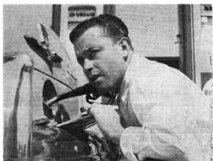
Gas mileage test without special instruments calls for extra care in filling tank, then noting level of fuel in pipe neck.
