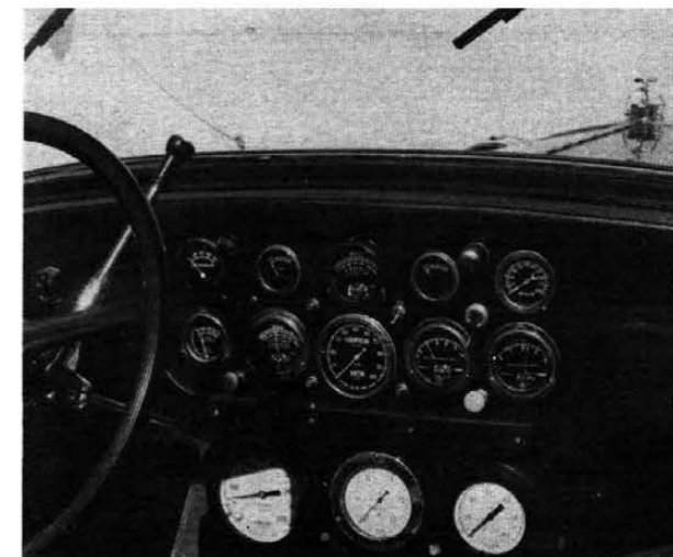
Dash panel of the Doble was a maze of instruments. Steam pressure gages are the white dials below the main dash.
