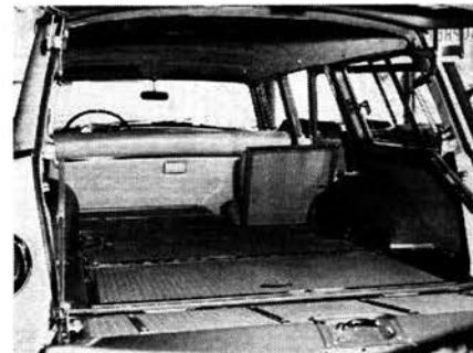
View from rear of Squire shows third seat removed. Note that only part of second seat can be folded down if so desired.
