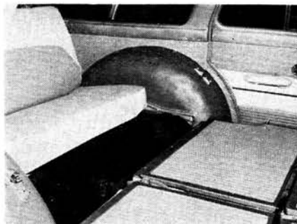
Converting interior of Country Squire and Country Sedan has many variations. Here middle seat folds down for cargo.
