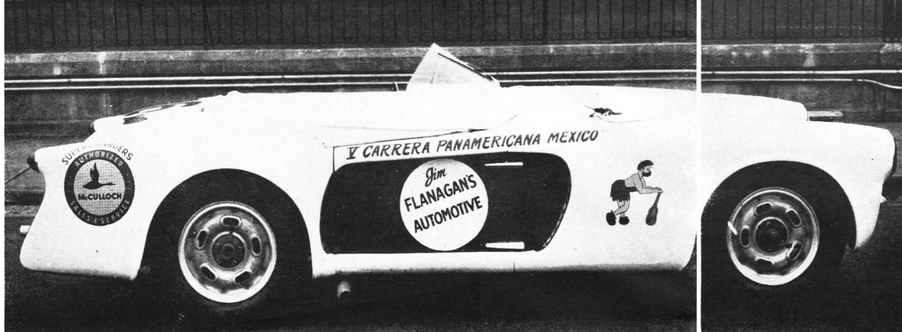
Kurtis still carries some of insignia used during 1954 race in Mexico, where the car was sidelined by overheating blamed on full belly pan. Although no stranger to road racing, the Nash engine is fairly uncommon in special cars.
