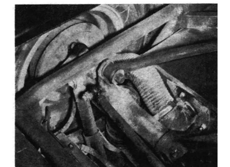
Air is fed to brakes through flexible tube. Coil spring, visible behind axle, has been added to handle heavy fuel load.
