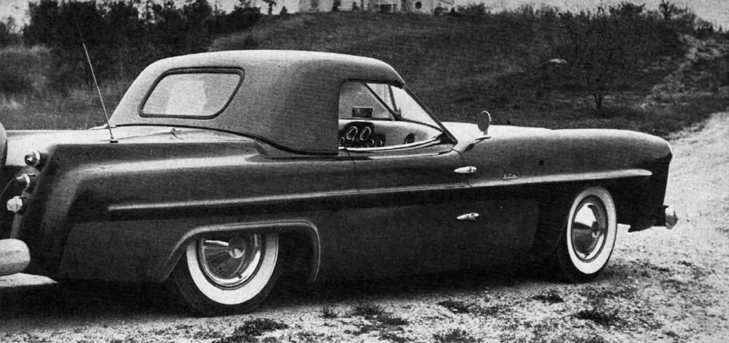
Sleek and sporty, La Saetta shown here with a detachable hardtop is only three feet high at the cowl. Body is fiberglass.
