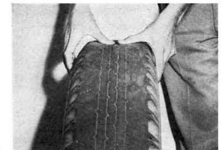
Tire for use on sand should be deflated to approximately six psi. In absence of gauge, softness is judged by one-in. flex.
