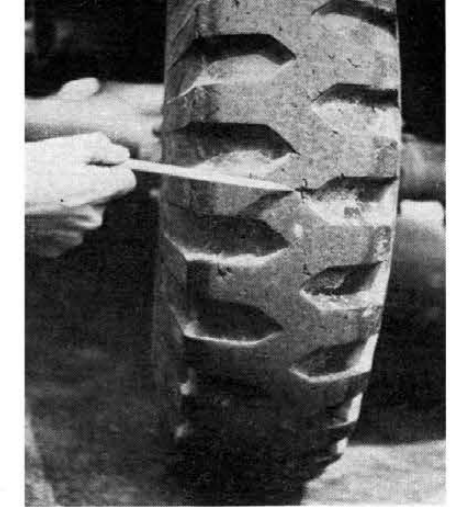
For rocky going, bar tread should be used since rocks would tear blocks from knobby treads. Cuts show the problem.
