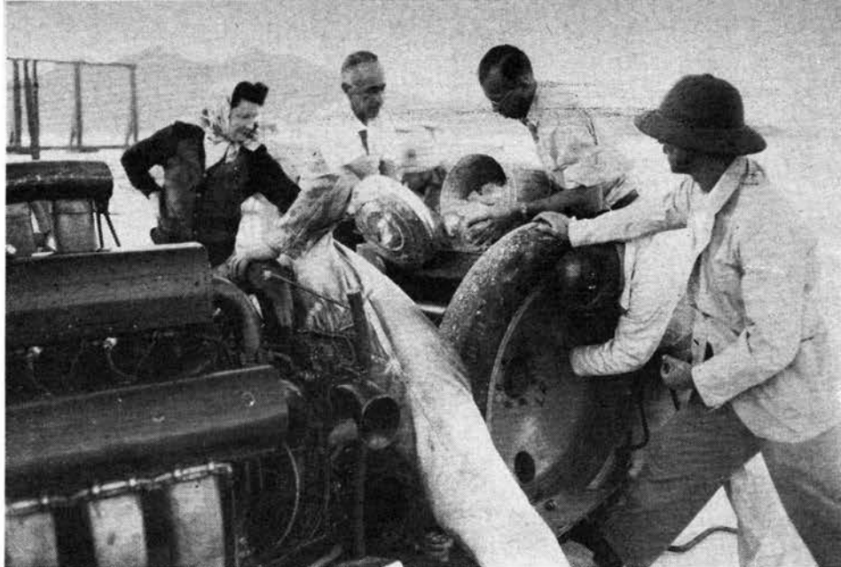
Ice is dumped into the cooling water tank, mounting a light-alloy disk wheel. The centrifugal blower and air intake are visible at the center of this pre-run photo.
