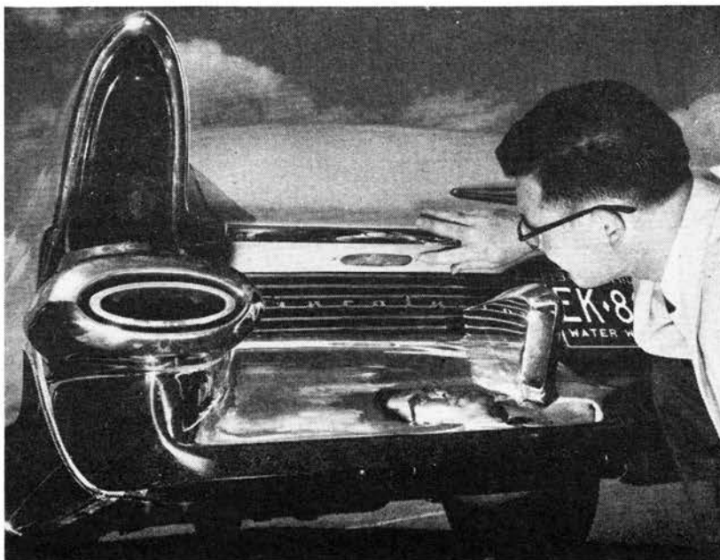
Backup lights are under rear deck ledge, with bumper serving as a kind of reflector. Huge dual exhaust outlet pipes are enclosed in pods on the bumper.
