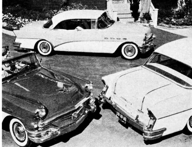
Super, top, Century, left, Roadmaster, right, share rear bumper with integral exhaust cutaway. Roadmaster deck strips, spear, letters distinguish it from others
