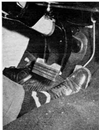
Doubly suspended big brake pedal suits itself to all driving techniques. Throttle is hanging, too
