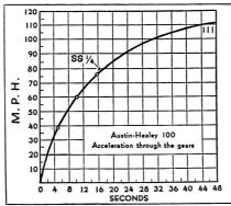
Specifications at a glance: Four cylinder, overhead valve engine; displacement—2660 cc; 90 bhp at 4000 rpm; wheel base—90 inches; curb weight 2150 lbs.; distribution 49%/51%; three forward speeds plus overdrive (synchromesh); steering 2½ turns lock to lock; brake area 145 square inches; average fuel consumption, 25 mpg.
