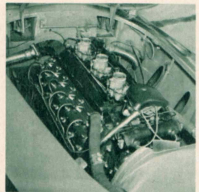
Left: the cockpit contains a large, sofa-seat and Stewart Warner instruments. Right: power is supplied by a '38 Packard V-12 with 3 Stromberg carburetors. Below: the all-steel body by Bohman & Sons, is mounted on a 105-in. wheelbase.
