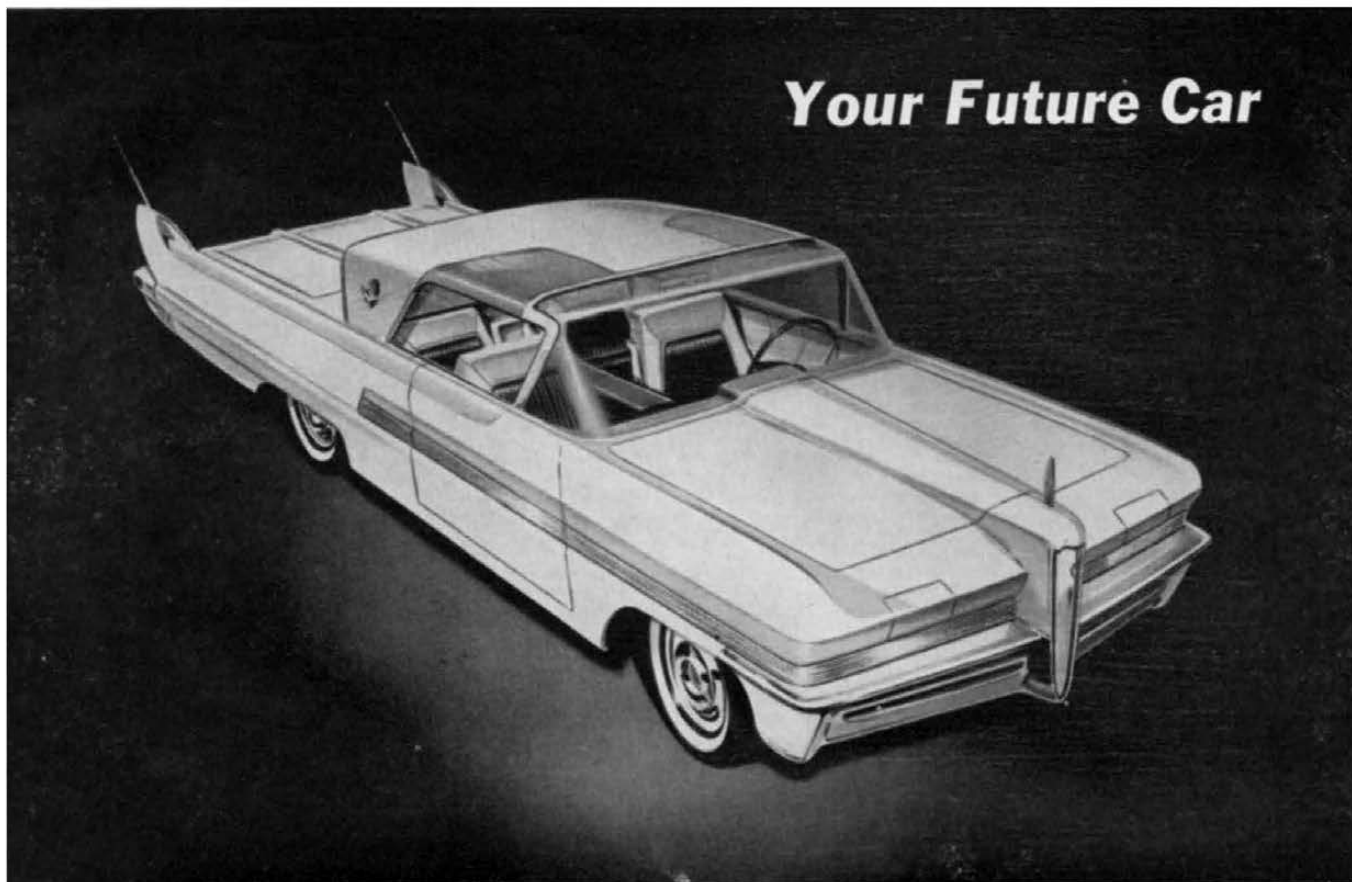
Packard's "Predictor" may not thrill the styling purist, but its chassis has a unit differential and transmission with independent rear suspension.
