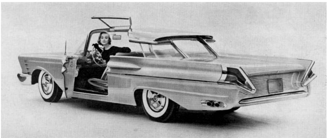
Mercury's new show car, the "XM-Turnpike Cruiser," has automatic "butterfly" door inserts in the roof, stands 52.8" high.
