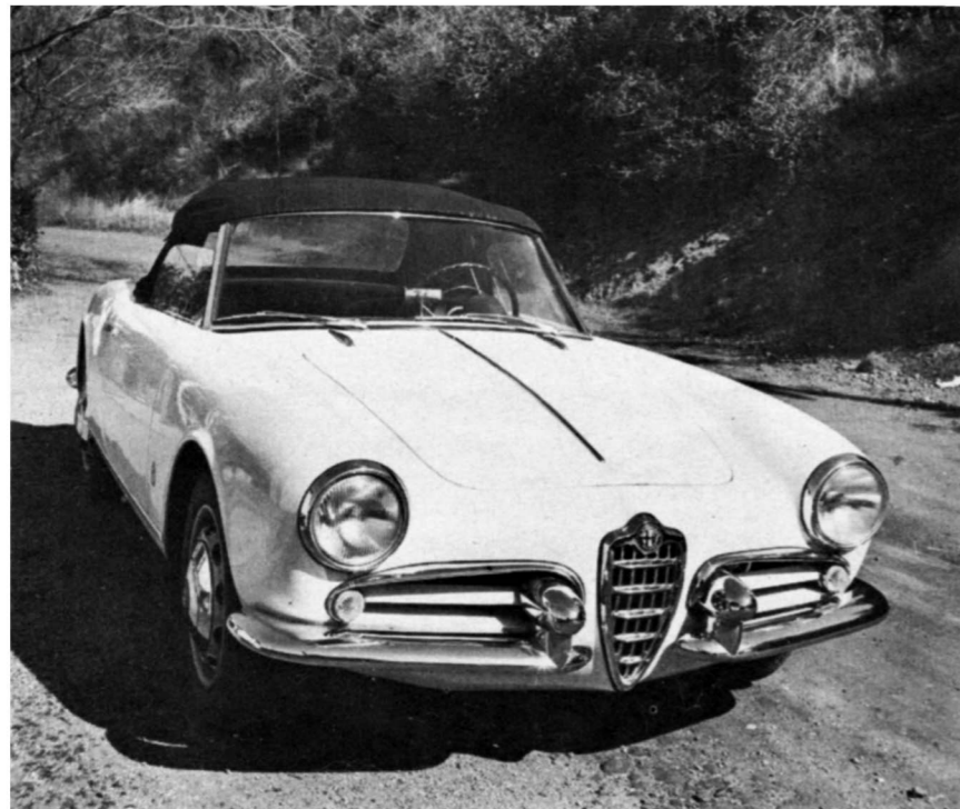
Three quarter front view shows the little Alfa's aerodynamic-type body. High beam is ultra-high, used in lieu of horn in Italy. This may be good for Quiet Week but illegal in U.S.
