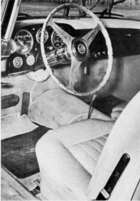
Instruments are placed directly before driver for quick spot checking. Adjustable steering column is reminiscent of Thunderbird.
