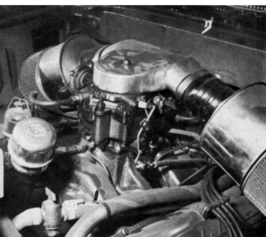
To keep hood height low, special double air cleaner is used. This is a standard Caddy engine. As is, stock power-to weight ratio is 12.1 to 1.
