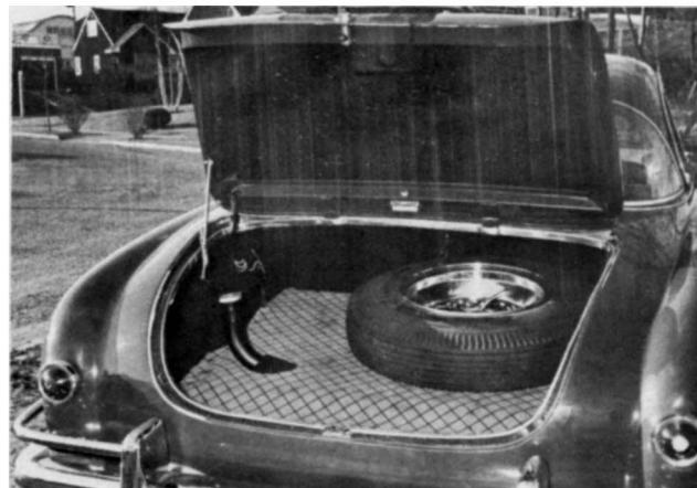
Trunk deck-lid is padded for sound absorption. Note the gas filler pipe inside the trunk. The inconvenience of opening the trunk to fill up is far outweighed by the smooth, uncluttered body lines.
