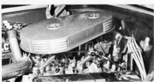
ABOVE: Dual Carburetors linked by one air cleaner are Carter four-barrel units. BELOW: Rear seat permits only two passengers to ride. Center rest is also small compartment. Courtesy light is under arm rest.
