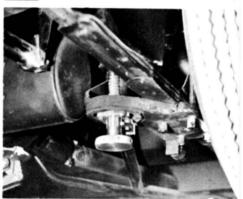
Apparently equipped with integral jacks at all four wheels.
