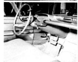
Instruments are set directly in front of driver. Note foot emergency brake. Deep dish wheel is padded.
