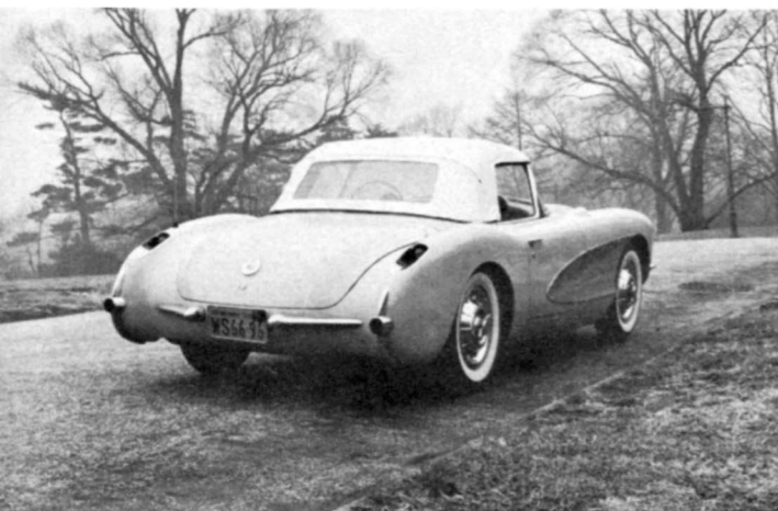
A lack of bumpers at the rear will make any Corvette driver over-cautious when backing. Exhaust tubes are in for abuse.
