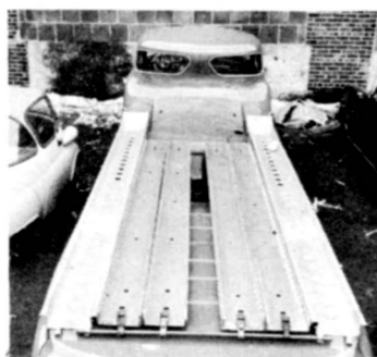
To cut down weight, channels are of light alloy material, and drilled. Tubular support carries weight of race car when loading for transport.
