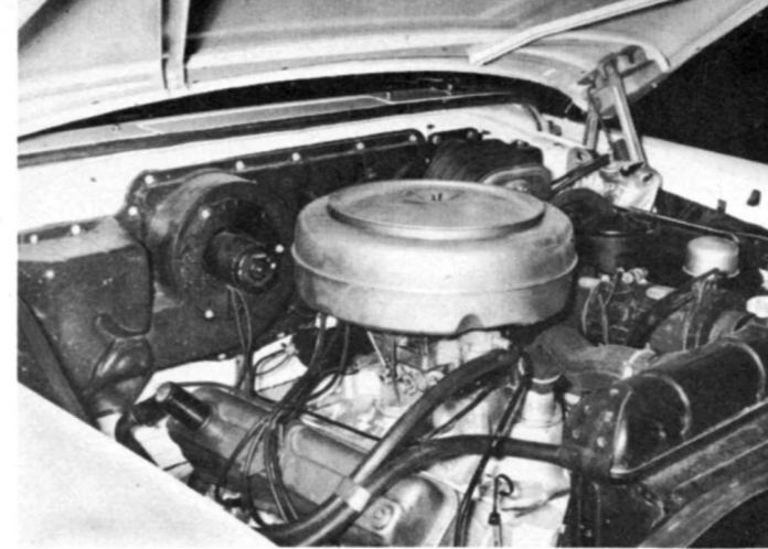
Cramped quarters under the hood leaves little room for the repairman to work efficiently. The high output V8 engine develops 240 bhp at 4800 rpm. Plymouth, mainly concerned with acceleration, worked on the low end of the scale for torque — 310 lbs.-ft at 2800 rpm.
