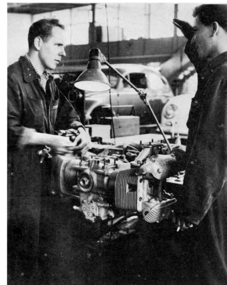
Assembling famed air-cooled Porsche engine, mechanics discuss details of work. Plant also handles production models scheduled for competition.
