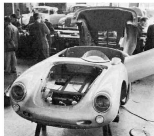
Front view of the Porsche Spyder. Battery and spare are carried here. Bulge on left fender is rear-view mirror.
