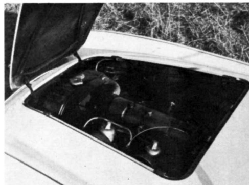
The 2660 cc engine sits snugly within the engine compartment. This little power-plant develops 90 bhp at 4000 rpm. Tight layout makes for some difficulty in minor service.
