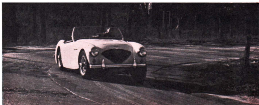
Cornering fast and hard, Austin-Healey-100 shows excess flexibility at the rear. This causes understeer on turns but gives little feeling of insecurity. Turn was taken at higher speed than would be normally advisable.
