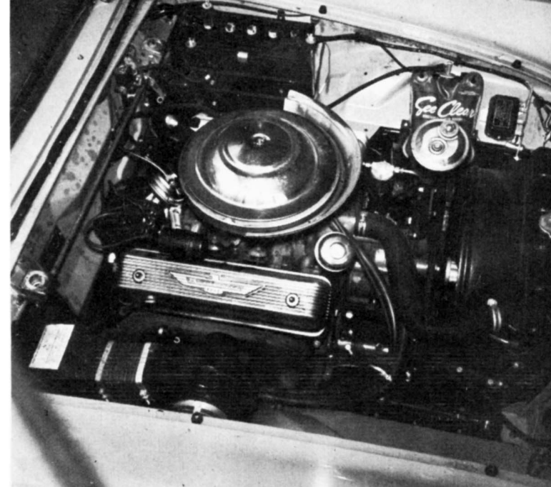
The power plant with the engine dressup kit. Underhood bright work costs an extra $21.50. This stock Fordomatic engine is rated at 225 hp.
