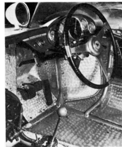
Unfinished cockpit of a Monza in assembly reveals polished light alloy interior. Early body designs were executed by Autodromo, Vignale and Farina, but later models owed their form and shape to Dino Ferrari, son of famous Enzo.
