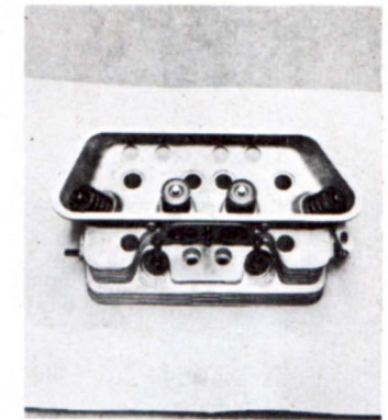
Top view of standard head. Note, deep and all around finning for optimum heat dissipation. Head is light alloy, easily removable.
