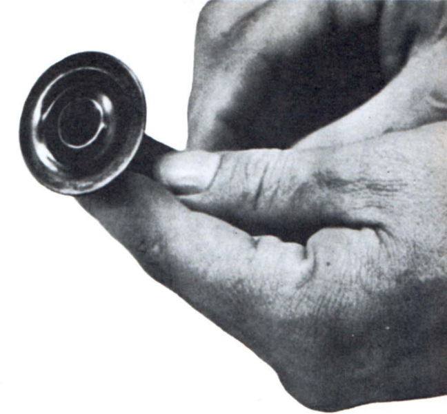
Exhaust valve has high center so that if piston strikes valve, it will close it, not bend stem.
