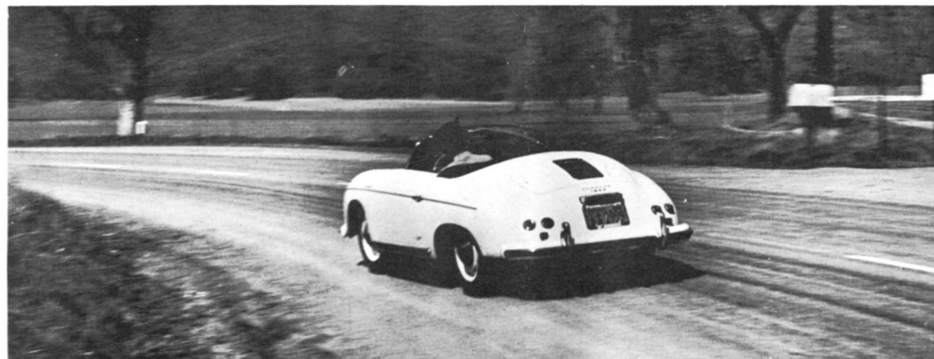
Porsche's tail slides toward outside of bend on standard test curve. This curve is not on a slope despite optical illusion, road is dead level. Car's driftability helps it achieve high average speeds.
