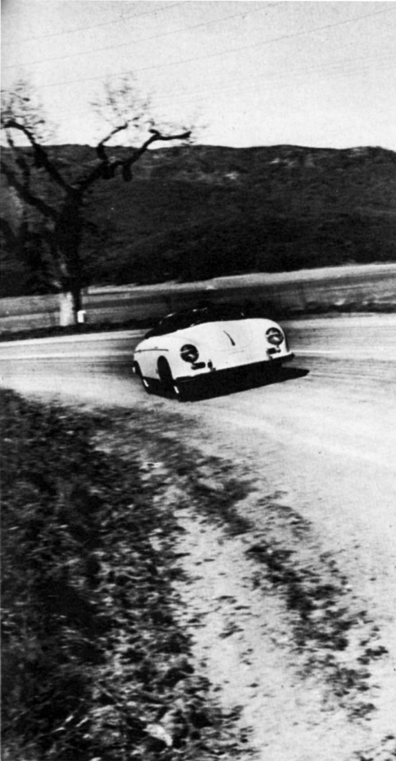
In moderate turns, the Speedster is slipped through under power all the way, directing the car by a combination of rear-wheel or four-wheel slip and throttle.
