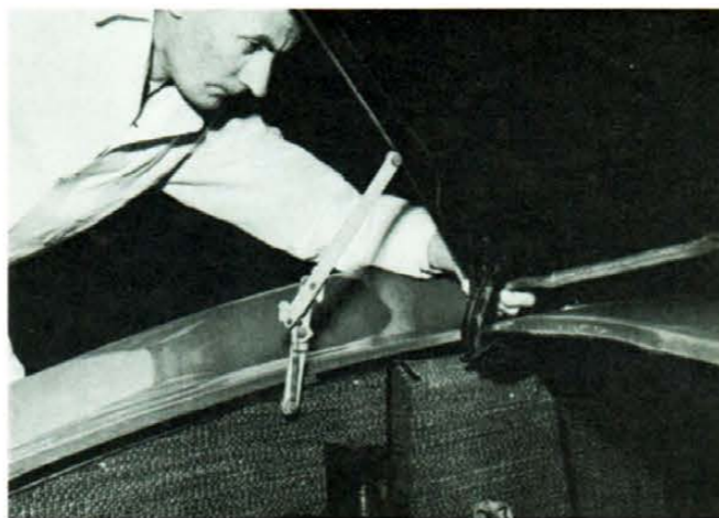
Trunk braces should be inspected for signs of repair. Welded braces could mean car has been in accident, which could also mean distorted frame.
