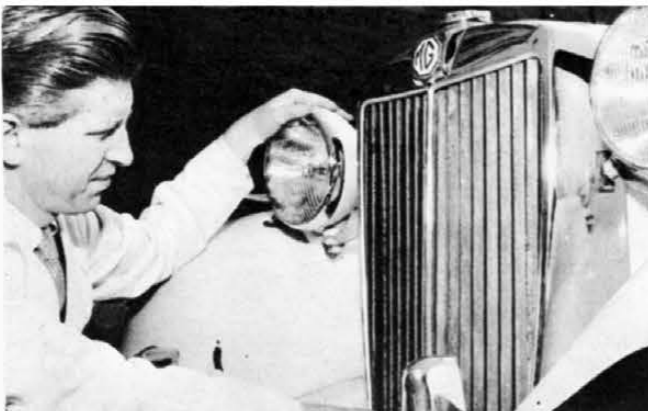
Chrome and grille parts should be checked for corrosion. Blistered chrome could mean the car has been outside in bad weather or near salt water.
