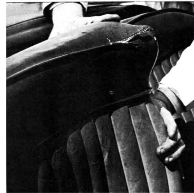
Worn or torn interiors denote either long hard use or perfunctory attitude toward maintenance of general appearance. Check list: fair to poor.
