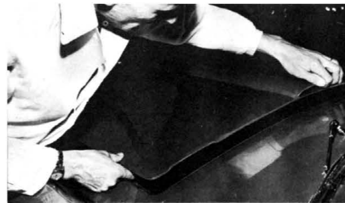
Inspect hood for proper alignment and action of hood hinges. These check points often reveal body racking or distortion due to collision. Check under-chassis for further evidence.
