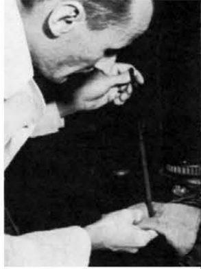
Inspecting dip stick reveals consistency of oil which may be heavy in order to muffle a slapping piston or a loose bearing. Also, if oil feels gritty between the fingers, a ring job may be in order.
