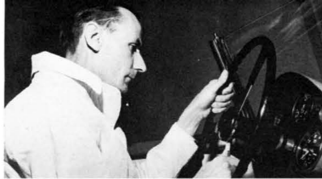
Test excessive play in steering box and linkage by rotating steering wheel slightly in both directions until front wheels are just laterally moved. If play exceeds inch and a half, have dealer repair it.
