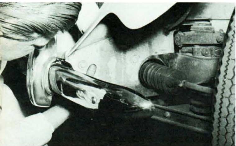
Signs of a front-end collision can be detected on the body metal behind the bumper brackets. Small points such as this are often overlooked by adept body shops.
