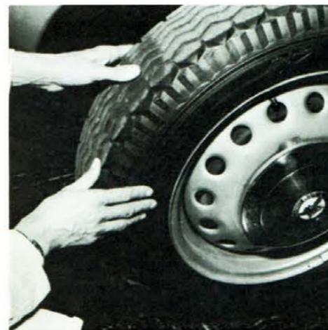
Scuffing, cupping or uneven wear on inner or outer perimeter of tread indicates bad alignment, or worn parts.
