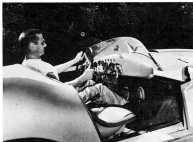
With excellent grouping of instruments, adjustable bucket seats, precise location of shift lever and handbrake, ample leg room for the lanky, the A-B cockpit leaves little to be desired.
