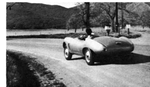
Weight distribution, and stable suspension geometry permit high cornering speeds with slight drift.
