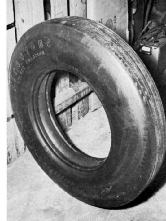
Firestone "Bonneville" tire used by Corvette at Daytona. Note thin tread layer and smooth side casing.
