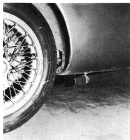
Borrani wire wheels carry either Pirelli or Dunlop tires. Note exhaust is deflected away from rear tires and into slipstream.
