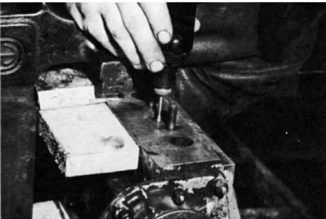
Using a small burr to clean intake ports, mechanic is careful not to dig through the thin walls.
