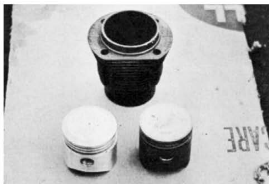
Special 80mm 7-1 piston on left slightly domed. Piston on right has concave head and a compression ratio of 5.8-1. Barrel is stock cast iron.
