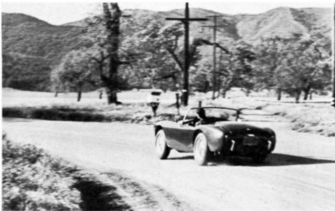
Leaving test bend, the Ace demonstrates its controllable slide which can be induced below 55 mph by using more throttle and deliberately pivoting car on front wheels. Curve-site is SCF's special test bend.
