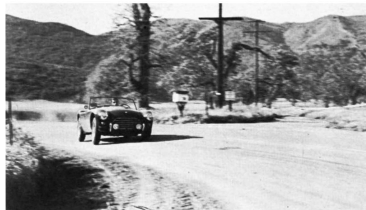
At 60 mph through test curve, the Ace leans hard, but remains glued to road. Good proportion of weight on rear wheels, and all around independent suspension makes this one of the best cornering cars tested.
