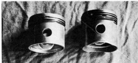
Merryman piston at left, A-H piston at right. Merryman piston is \frac{1}{16} shorter in wrist-pin height, has unrelieved skirt.
