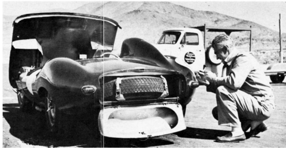
In compliance with FIA regulations, The Jag carries its spare in a readily accessible location. On long races, quick changes can be essential in case of tire failure.
