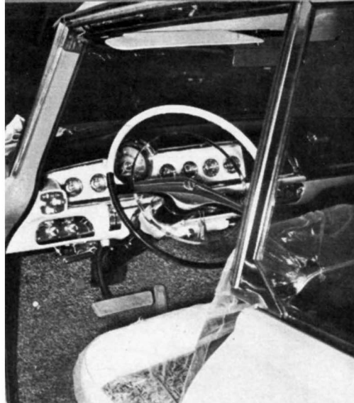
Instrument panel layout is easy to read with speedometer located in driver's line of vision. Note wide brake pedal, to be operated with either foot.
