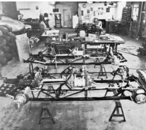
Twin Novi chassis in the final stages of completion. Engines are last to be installed. Note long, heavy tubular drag link to steering idler arm.
