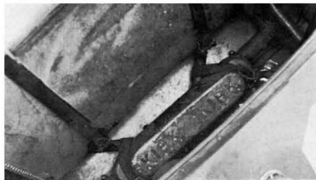
To make the rear wheels stick to the tight course, 100 lb. lead bar was strapped to frame of ex-Fangio Ferrari. Car still broke loose.
