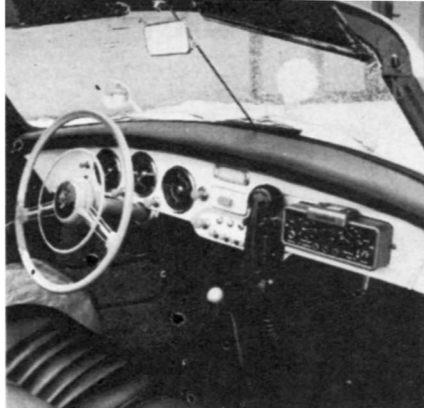
Two way short wave radio is part of the latest equipment of the Autobahn Police. Switches and dials of unit set neatly in the glove compartment.
