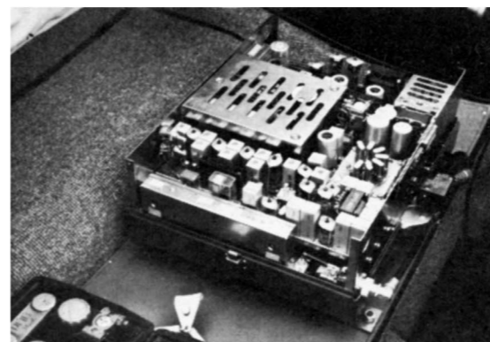
Combined transmitter and receiver unit sits behind driver and assistant. Two six volt batteries connected in series power the short wave set.
