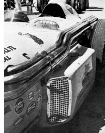
Agajanian car was exhaust tuned by Frank McGurk. Tuning was too efficient, scavenging intake. It was replaced.
