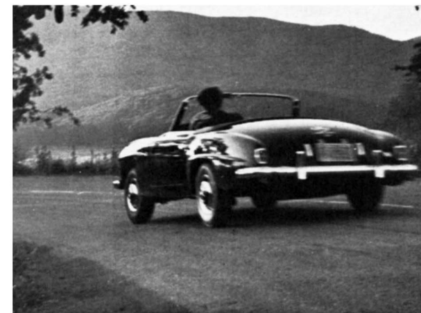
Here the car takes the test curve at 60 mph. There is almost no roll to the body giving it a flat ride. It has that well-braced feeling in corners.
